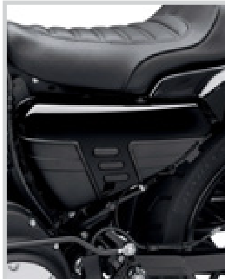
C. CUT BACK BATTERY COVER
