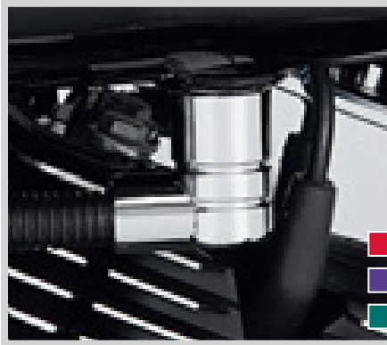
F. FUEL TANK FITTING COVER
