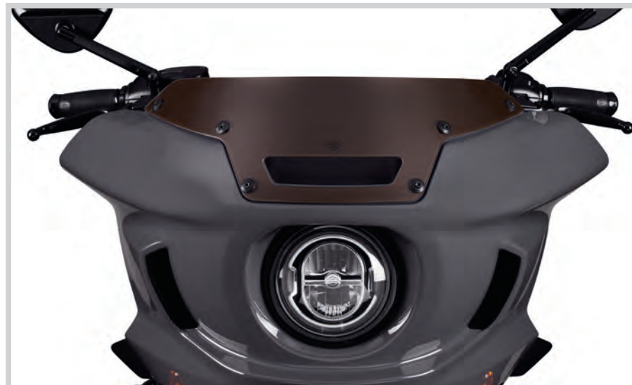
C. ST WIND DEFLECTOR
