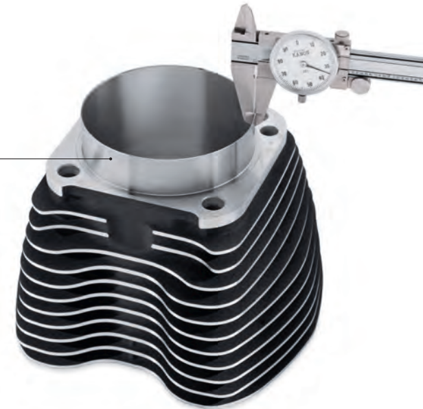
HIGH-STRENGTH CYLINDER LINERS ARE MACHINED TO SLIP INTO THE STOCK CASE OPENING
