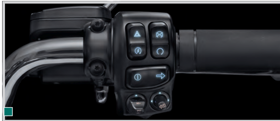
B. LIGHTED HAND CONTROL SWITCHES
