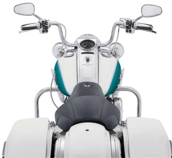
**Figure 2-46. ROAD KING® / ROAD GLIDE® REACH® HANDLEBAR****Table 2-500. Note****ALL MODELS**
