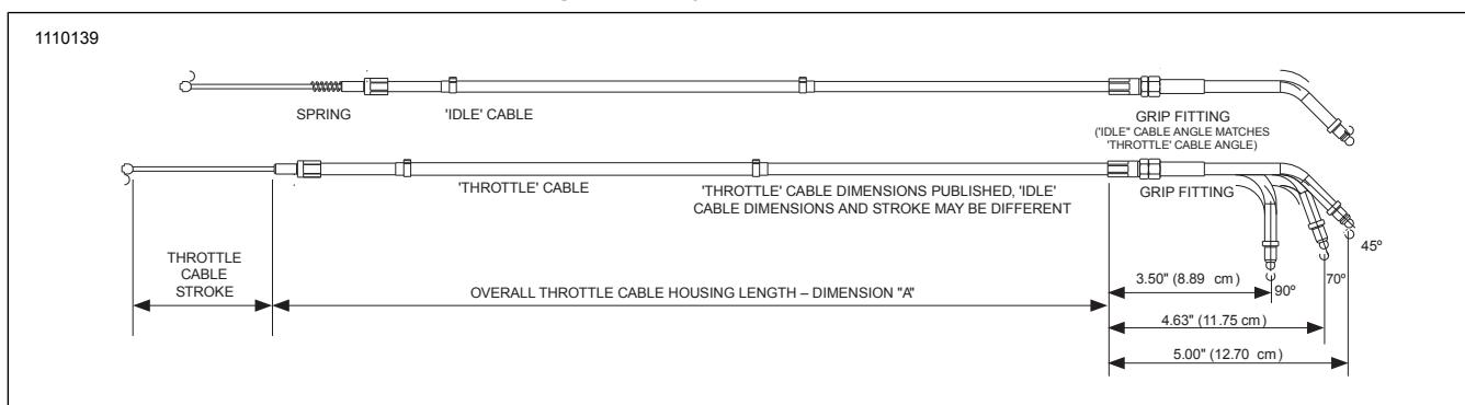
**Figure 3-4. Throttle/Idle Cables**
