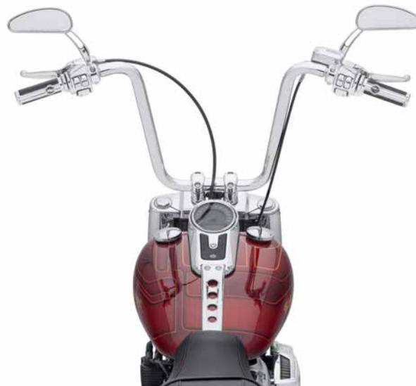
**Figure 2-19. 16" FAT APE HANDLEBAR KIT WITH RISER****Table 2-147. Note****ALL MODELS**
