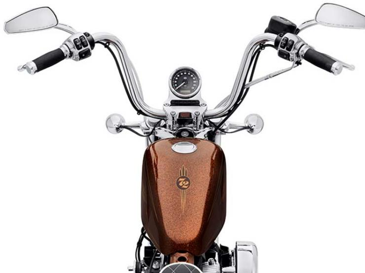
**Figure 2-8. MINI-APE HANDLEBAR****Table 2-33. Note****ALL MODELS**
