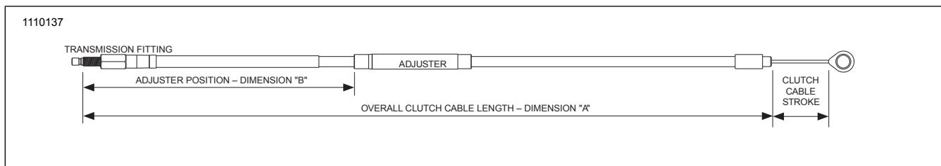
**Figure 3-2. Clutch Cables**
